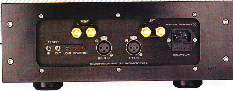
ABOVE: Balanced (XLR) inputs and screw-down speaker terminals. The close setting of the latter and surrounding metal casework means great care should be taken with bare speaker cable and/or 4mm spade adapters
